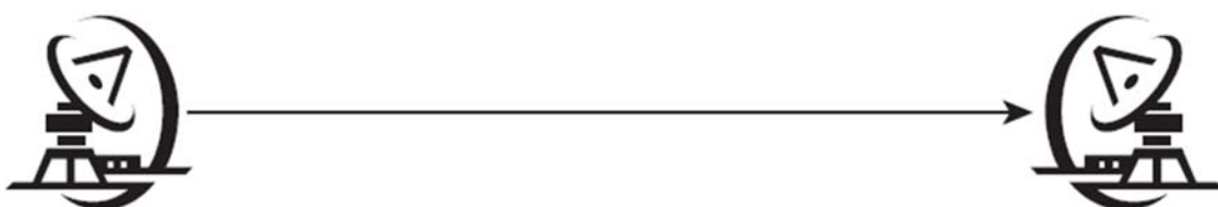
Directional Antennas and Line of Sight
