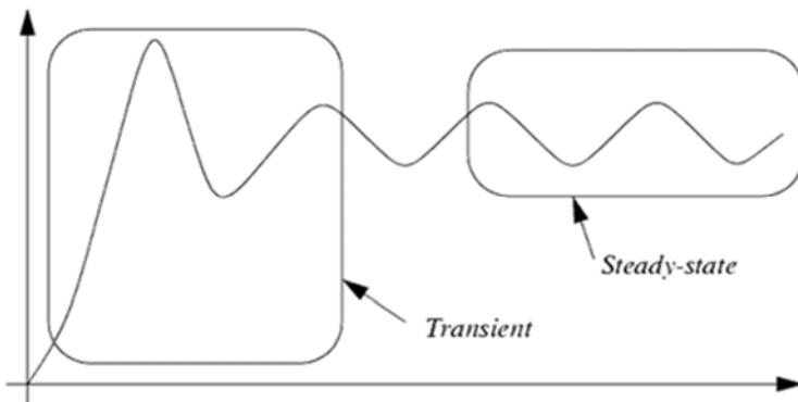
Note: the transient response is predicted with the homogeneous solution. The steady state response is mainly predicted with the particular solution, although in some cases the homogeneous solution might have steady state effects, such as a non-decaying oscillation.
