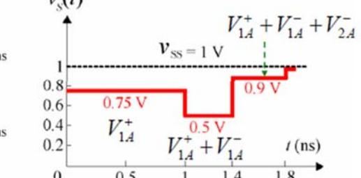
$$\begin{array}{ll} \Gamma_L = 0.6 & \Gamma_S = 0 \\ \Gamma_{BA} = \frac{1}{3} & \Gamma_{AB} = -\frac{1}{3} \\ T_{BA} = \frac{2}{3} & T_{AB} = \frac{4}{3} \end{array} \quad \begin{array}{ll} Rs = 50 & Rl = 100 \\ Za = 50 & Zb = 25 \end{array}$$
