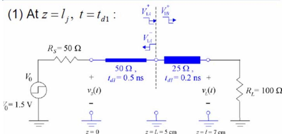
$$v_{1A}^+(l_j, t_{d1}) + v_{1A}^-(l_j, t_{d1}) = v_{1B}^+(l_j, t_{d1})$$
