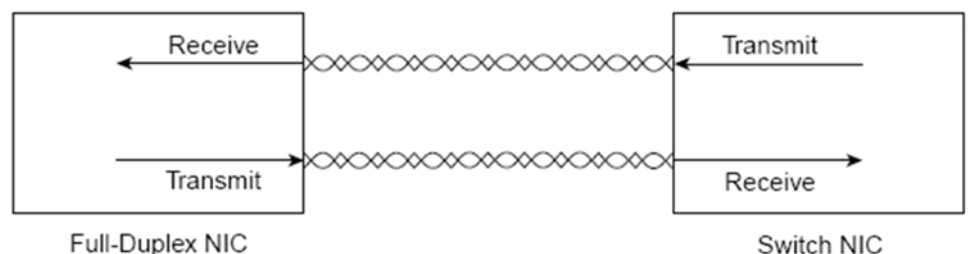
10BASE-T Full-Duplex Operation Using a Switch
