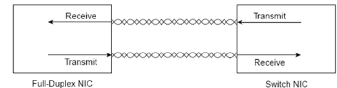
10BASE-T Full-Duplex Operation Using a Switch
