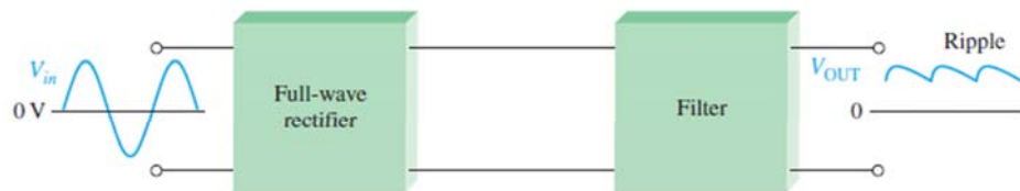
(b) Rectifier with a filter (output ripple is exaggerated)
