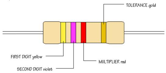
It is important to note that the physical size of the resistor indicates its power dissipation rating, not its ohmic value.
